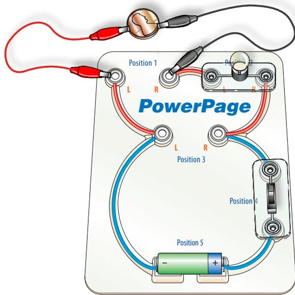
**STEP 7:** Attach the alligator clips to a penny. Does the lamp light up? **Yes.** Is the penny a conductor or insulator? **Conductor, the outside of a new (since 1982) penny is copper and the inside is zinc.**
